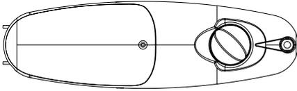
Place it in a central position to set an optimal temperature for normal use. The more you turn the knob clockwise, the lower the temperature in the refrigerator will be. The more you turn the knob counterclockwise, the higher the temperature in the refrigerator will be.
