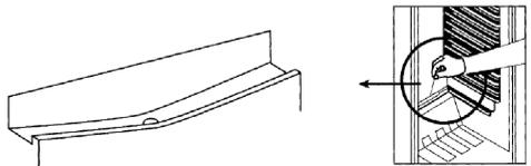
Make sure that the drain gully and the drain opening are not blocked so that the water
