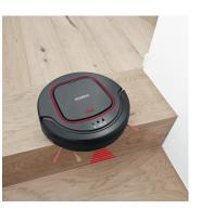
Intelligent: Stair step detection through modern sensor technology.
